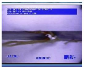
FIG A6.3: Example of an obstruction within a joint - not acceptable
