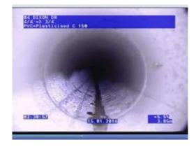
FIG A1.4: Example of poor quality footage of a joint - not acceptable
