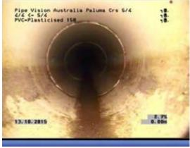
FIG A8.1: Example of a clean pipe - acceptable
