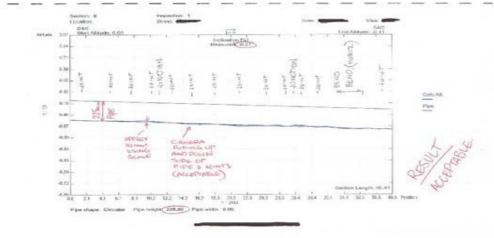
FIG A3.1: Example of how to review an inclination report – pipe acceptable
