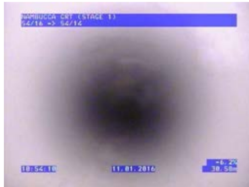
FIG A1.2: Example of poor quality footage – not acceptable
