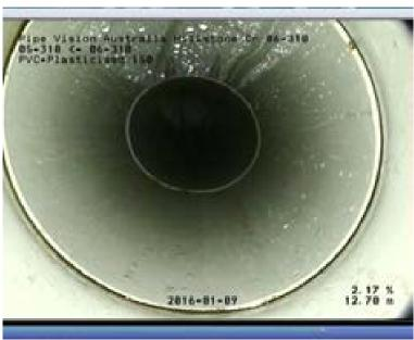
FIG A4.2: Example of deformation (ovality) - not acceptable
