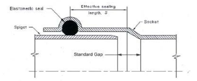
Adjusted Figure 7.1 from AS/NZS1260 showing the "Standard Gap" that is defined in the following Table:
