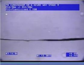
FIG A5.11: Example of no gap at a coupling - not acceptable
