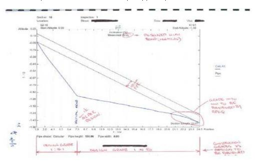
FIG A3.2: Example of how to review an inclination report – consulting engineer (RPEQ) to determine if acceptable
