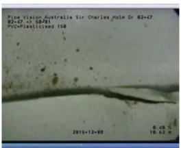
FIG A5.3: Example of a defect at a joint - not acceptable
