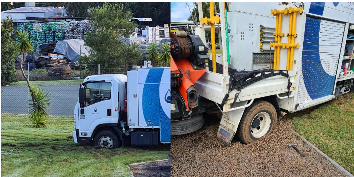
Figure 24. Soft surfaces can be problematic for trucks accessing tanks and wells.
